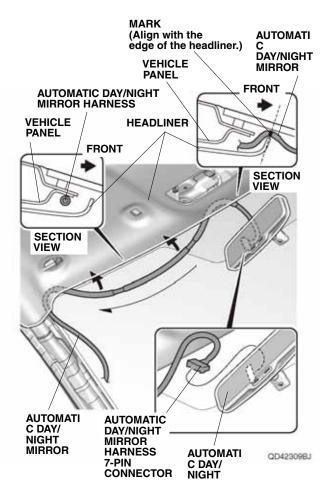
24. Gentry pull back the headliner, and tuck the automatic day/night mirror harness behind the headliner. Align the mark on the automatic day/night mirror harness with the edge of the headliner. Be careful not to crease the headliner.
