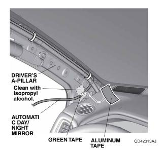
29. Attach the green tape on the automatic day/night mirror harness to the driver's A-pillar with one aluminum tape.
