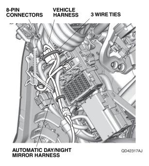
34. Route the automatic day/night mirror harness along the vehicle harness. Remove the bolt, and install the automatic day/night mirror harness ground terminal with one ground bolt.
