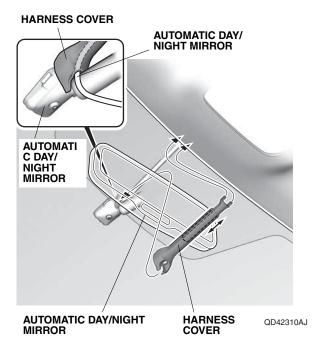
26. Route the automatic day/night mirror harness down the A-pillar as shown. Align the green tape on the automatic day/night mirror harness with the vehicle clip, and secure the automatic day/night mirror harness to the vehicle harness with two wire ties. Do not cover the installation holes of the driver's A-pillar trim.
