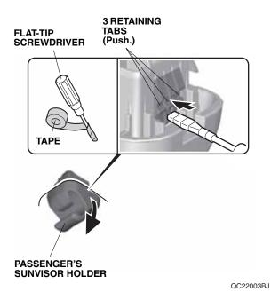
While holding down the passenger's sunvisor holder as shown, use a flat-tip screwdriver wrapped with a tape to remove the passenger's sunvisor holder (three retaining tabs).
