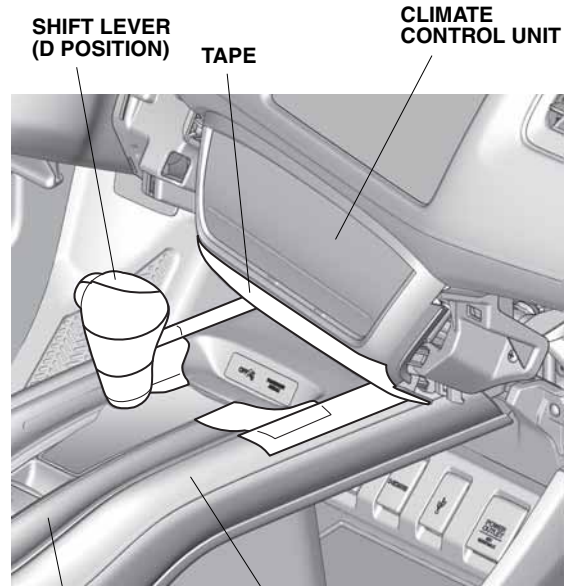
SHIFT LEVER (D POSITION) TAPE CLIMATE CONTROL UNIT CENTER CONSOLE PANEL CENTER CONSOLE PAD QD41602AJ
