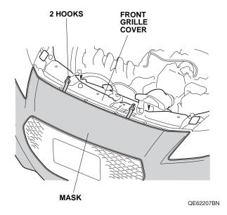
14. Close the hood, and adjust the position of the mask to the hood.
