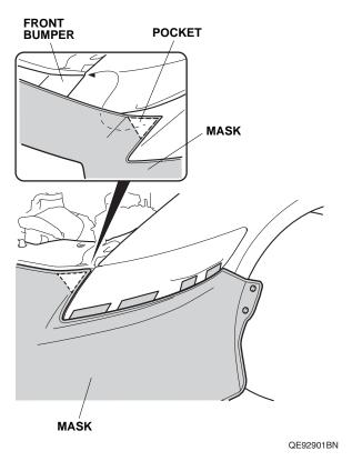
6. Pull the mask back toward the left front inner fender, smooth out any wrinkles, and secure two snaps on the mask to the two snap-screws.
