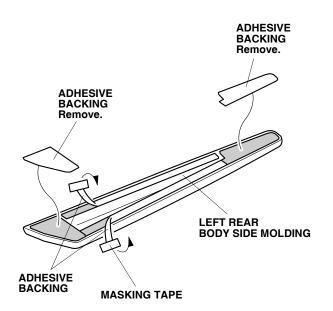
10. Align the left rear body side molding with the rear template, and attach it to the body panel.
