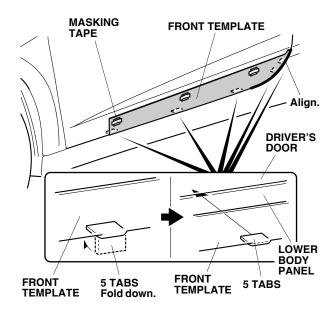
4. Align the front template to the driver's door and attach it with masking tape.
