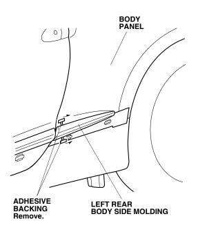
15. Using a rubber roller, apply pressure against the body side molding and roll from one end to the other.
