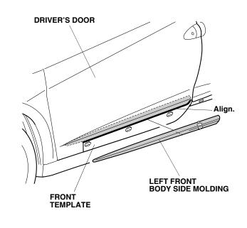
Peel back approximately 1½ to 2 inches of adhesive backing from each adhesive strip, and tape the ends to the front surface of the body side molding. Remove the end pieces of the adhesive backing.
