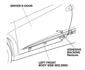
13. Using a rubber roller, apply pressure against the body side molding and roll from one end to the other.
