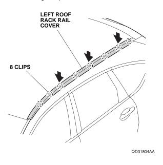
17. Secure the left roof rack rail cover to the left roof rack base with one self-tapping screw.
