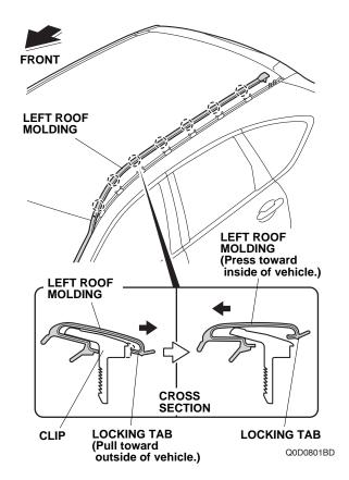
4. While pulling up the left roof molding, remove the two clips. Insert the plastic trim tool alternately to each slots in the clip, and release the locking tabs in the order shown. When removing the left roof molding, start from the rear of vehicle and work towards the front. Be careful not to deform the roof molding.
