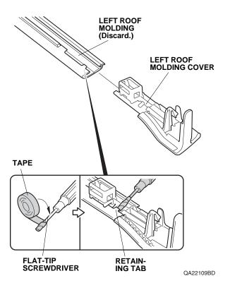
13. Reinstall the left roof molding cover in its original position on the roof.
