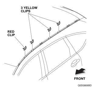
12. Using a flat-tip screwdriver wrapped with tape, remove the left roof molding cover from the left roof molding (one retaining tab). Discard the left roof molding.
