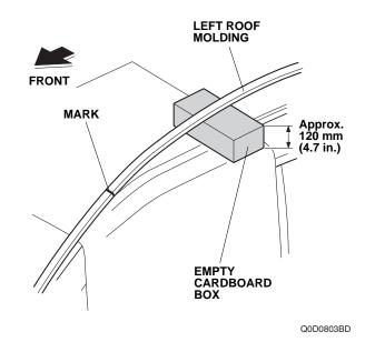
7. While wearing an eye protection, use an air saw to cut the left roof molding at the mark. Do not use a cutting wheel or shears to cut the left roof molding, it will damage the left roof molding. Have an assistant hold the rear edge while cutting.
