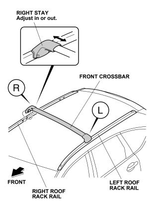
3. Secure the front crossbar to the roof rack rails using four bolts. Torque the bolts to 10 N·m (7.3 lbf·ft).
