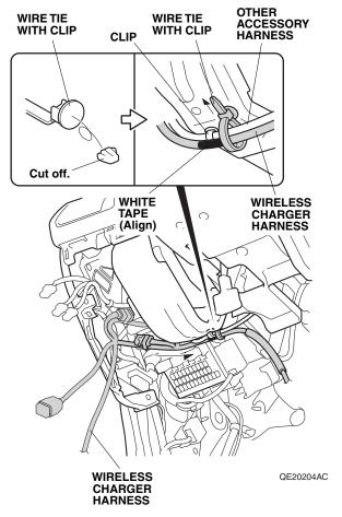
36. Attach the cut wire tie with clip around the white tape on the wireless charger harness and secure the wireless charger harness to the other accessory harness with one wire tie with clip.
