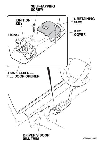
5. Remove the self-tapping screw from the trunk lid/fuel fill door opener cover.
