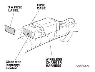
26. Using isopropyl alcohol on a shop towel, thoroughly clean the area where the urethane tape will attach.
