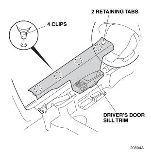
2-Door: Two retaining tabs and six clips.
