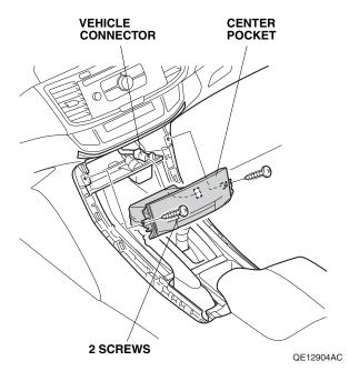
19. Open the armrest, remove the center console panel, and unplug the vehicle connectors.
