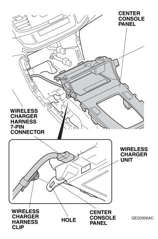
45. Secure the wireless charger harness to the center console panel with one clip on the wireless charger harness. Install the center console panel.
