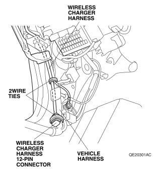
40. Align the white tape on the wireless charger harness with the vehicle clip and secure the wireless charger harness to the vehicle harness with one wire tie.
