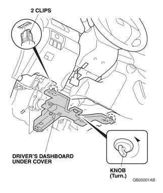
3. Remove the driver's dashboard lower cover and unplug the vehicle connectors.
