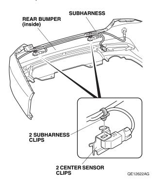
16. Using isopropyl alcohol on a shop towel, thoroughly clean the rear bumper where the aluminum tape will attach.
