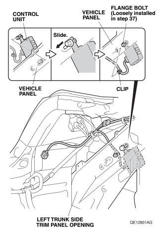
40. Secure the clip on the backup sensor harness to the vehicle panel.
