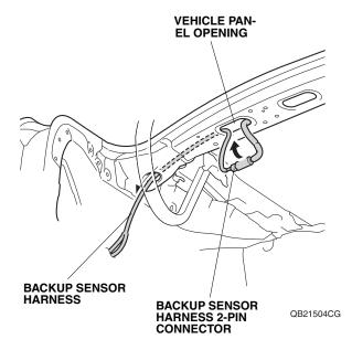
29. Secure the backup sensor harness to the vehicle harness with one wire tie.
