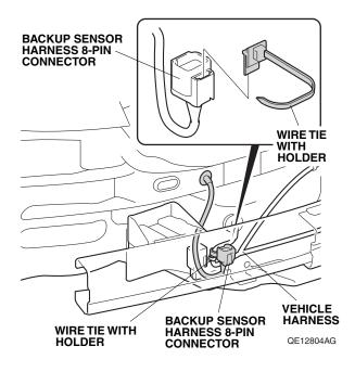
46. Install the connector clip on the backup sensor harness 8-pin connector, and secure it to the vehicle panel.
