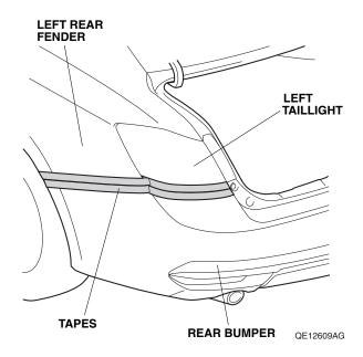
Remove the two bumper screws, four self-tapping screws and six clips.
