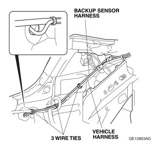
45. If equipped with vehicle harness, install the wire tie with holder on the backup sensor harness 8-pin connector, and secure it to the vehicle harness. Go to step 47.
