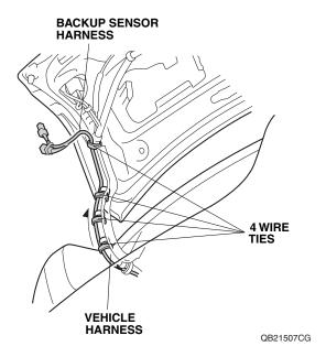
33. Unplug the vehicle 2-pin connector (Green) from the left backup light, and plug it into the backup sensor harness 2-pin connector.
