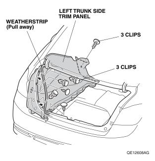
7. If equipped, remove the trunk panel.
