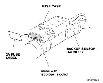
26. Route the backup sensor harness as shown, and plug the backup sensor harness 2-pin connector into the buzzer harness 2-pin connector.
