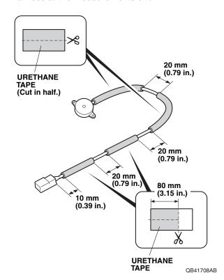
Using scissors, cut one urethane tape into three pieces. Wrap the two cut pieces of urethane tape around the buzzer harness at the measurements shown. 20. Route a piece of steel wire through the trunk area as shown.
