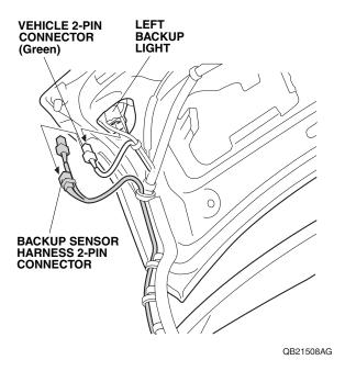
34. Plug the backup sensor harness 2-pin connector into the left backup light.
