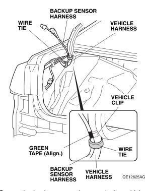
31. Secure the backup sensor harness to the vehicle harness with one wire tie.
