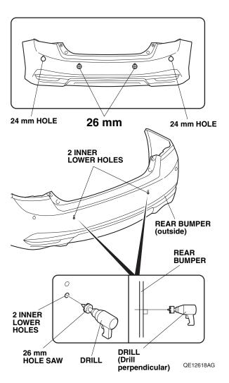
12. Using the two center sensor clips, install the two center sensors (Blue) into the 26 mm holes in the rear bumper. Note the direction and the pin location for each sensor.
