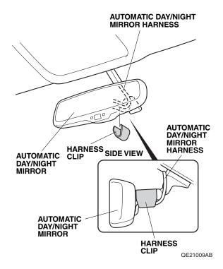
40. Secure the automatic day/night mirror harness to the vehicle harness with two wire ties as shown.
