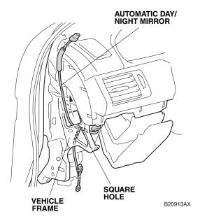
28. Secure the automatic day/night mirror harness to the vehicle harness with one wire tie as shown.
