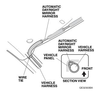
36. Plug the automatic day/night mirror harness 7-pin connector into the automatic day/night mirror.
