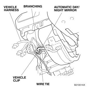
29. Route the automatic day/night mirror harness ground terminal toward the vehicle ground terminal.
