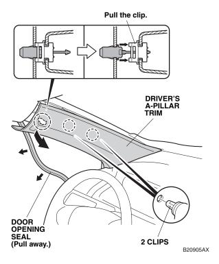
10. Pull out the driver's A-pillar trim to release the clips.
