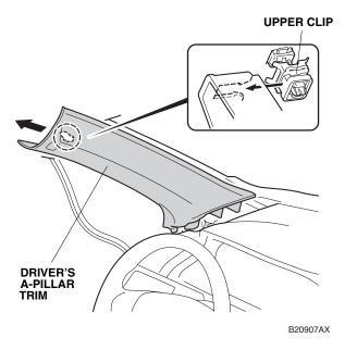
13. Remove the remaining upper clip from the driver's A-pillar.
