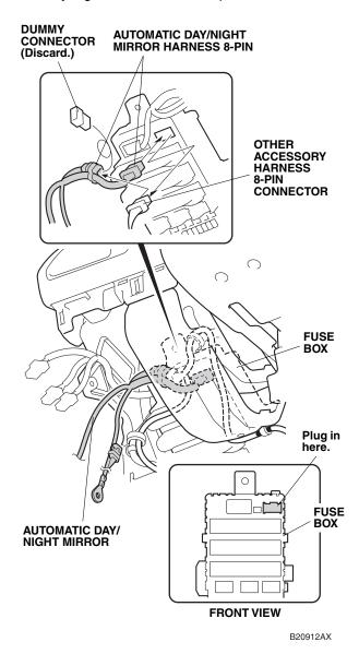
27. Route the automatic day/night mirror harness out of the square hole, and toward the outside of the vehicle as shown.
