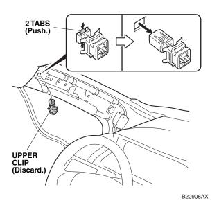
14. Install the new clip (supplied) on the driver's A-pillar trim, but do not reinstall the trim at this time.
