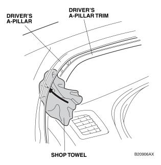
12. Slide the driver's A-pillar trim up to remove it from the upper clip. Carefully remove the shop towel and any clips that fell from the driver's A-pillar trim.
