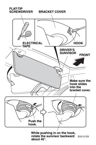
7. While pushing in on the hook, rotate the driver's sunvisor backward about 45°. Make sure the hook slides into the bracket cover.
