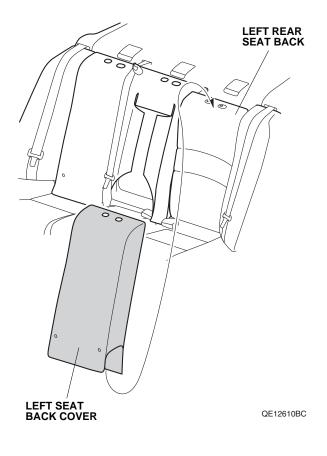
12. Secure the fastener on the left rear seat back. Raise the left rear seat back and lock it to its original position.
