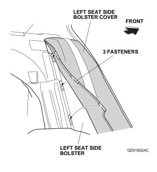
7. Insert the two tabs to the left seat side bolster.
