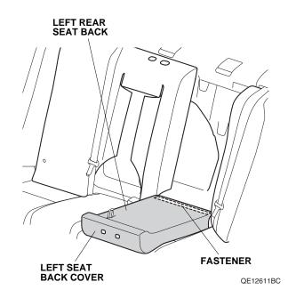
13. Insert each seat back cover under the head restraint guides. Pull down the armrest, and secure the three fasteners on the right rear seat back.
