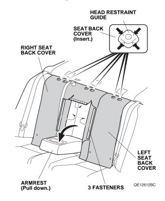
14. Insert the seat back covers between the rear seat backs and the rear seat cushion, and secure the three fasteners to the rear seat backs.
