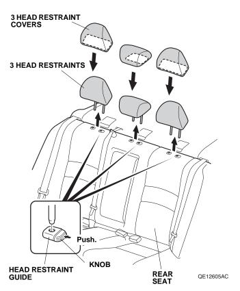
2. Fit the three head restraint covers over the head restraint.
