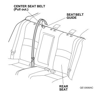
4. Open the trunk. Pull the levers, and fold the rear seat backs forward.
