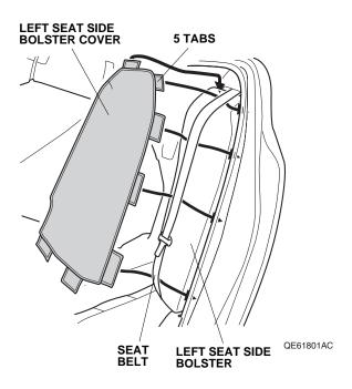
6. Secure the three fasteners to the left seat side bolster.
