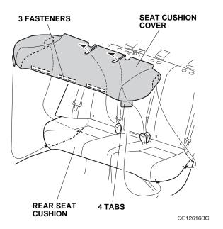
19. Insert the seat cushion cover between the rear seat back and the rear seat cushion, and secure the three fasteners to the rear seat cushion.
