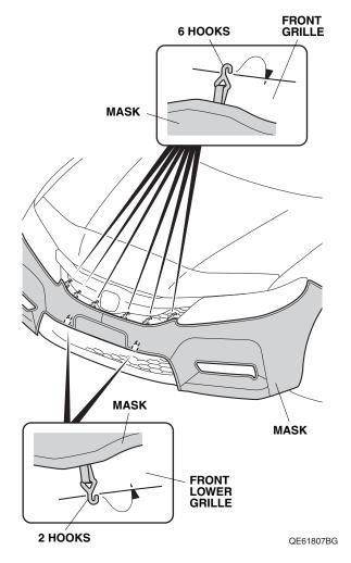
11. Attach two hooks to the inside edge of the front lower grille.
