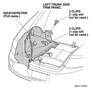
6. Remove the right trunk side trim panel the same way. **Installing the Anchors**
