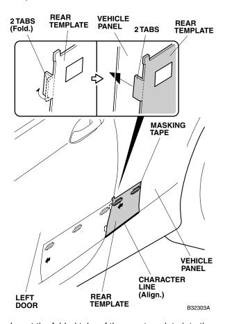
Insert the folded tabs of the rear template into the opening between the left door and the vehicle panel.
