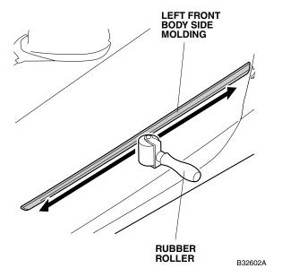
12. Peel back approximately 38 to 50 mm (1.5 to 2.0 in.) of adhesive backing from each adhesive strip, and tape the ends to the front surface of the body side molding. Remove the small end pieces of the adhesive backing.
