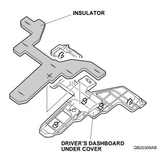
21. Install the ambient light to the driver's dashboard under cover as shown.
