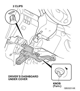
4. Remove the driver's dashboard lower cover (nine clips and unplug the vehicle connectors).
