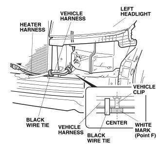
19. Secure the heater harness to the vehicle harness with one additional black wire tie.
