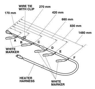
8. Using a white marker, mark the heater harness at each measurement shown.
