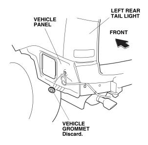
43. Route the backup sensor harness through the vehicle grommet hole, and install the backup sensor harness grommet to the vehicle panel. Make sure to install the grommet in the correct orientation. Do not pull on the backup sensor harness when installing the grommet.
