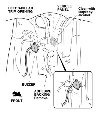
27. Route the buzzer harness along the vehicle harness, and secure it to the vehicle harness with one wire tie.
