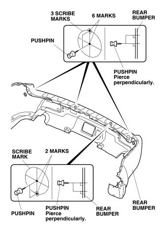
56. While wearing eye protection, drill the eight pierced marks with a 3 mm drill bit from the painted side of the rear bumper.
