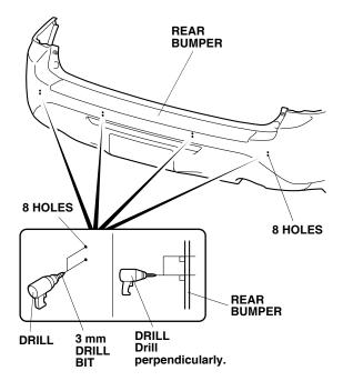
57. While wearing eye protection, enlarge the two *lower 3 mm outer* holes to 24 mm using a 24 mm hole saw.
