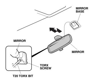
8. Install the automatic day/night mirror on the mirror base as shown, and tighten the Torx screw.
