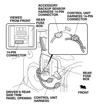
Plug the accessory backup sensor harness 14-pin connector into the control unit harness 14-pin connector. 20. Plug the control unit harness 14-pin connector to the 14-pin opening in the rear fuse box.
