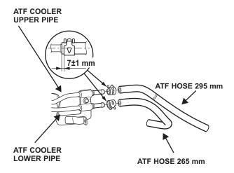
60. Route the hoses installed on the ATF cooler through the hole cut in the left air guide, and fit the ATF cooler into place on the bulkhead. Install the three washerbolts from the kit through the ATF cooler into the threaded holes in the front bulkhead. Tighten the bolts securely.
