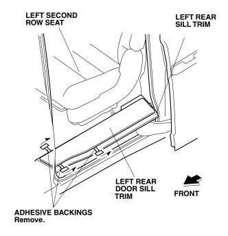
22. Using a rubber roller, apply pressure against the left rear door sill trim and roll from one end to the other.
