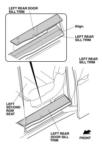
21. While applying light pressure against the left rear door sill trim, carefully remove the three adhesive backings.
