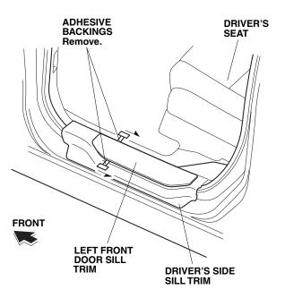
Using a rubber roller, apply pressure against the left front door sill trim and roll from one end to the other.
