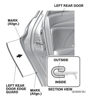
14. Starting at the upper side, use a rubber mallet to tap the left rear door edge guard into position with a series of light taps, then work down. Once in place, do not attempt to remove, reposition, or reinstall the left rear door edge guard.
