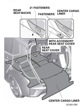
6. Position the center cargo liner in the cargo area, and secure it with seven fasteners.
