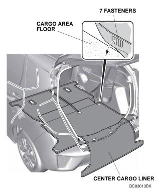
7. Secure the outer two fasteners on the center cargo liner to the fasteners on the left and right cargo liners.
