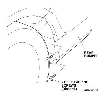
Install the left rear splash guard onto the rear bumper with two self-tapping screws, and tighten them in the order shown.
