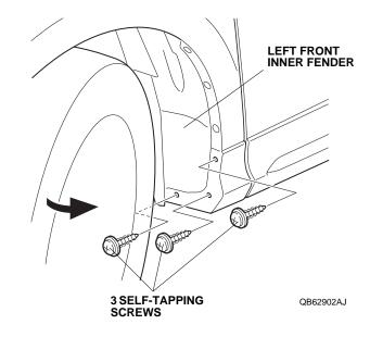
2. Remove three self-tapping screws from the left front inner fender.
