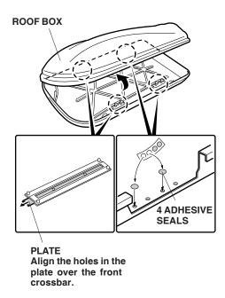
3. Attach adhesive seals over the unused rear mounting holes in the bottom of the roof box. The seals will help prevent water from entering the roof box. Remove the roof box from the vehicle.
