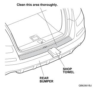
5. Using a spray bottle with 3M protective tape application solution, spray the area where the rear bumper applique will attach. Spray some solution on your hands.
