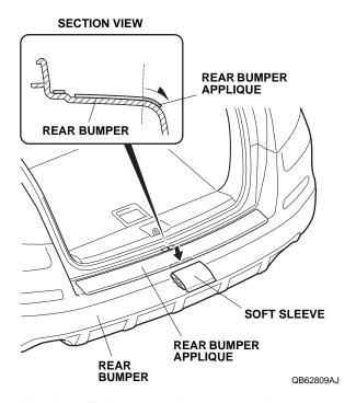
14. Use the soft sleeve to adhere the rear bumper applique to the lower section as shown.
