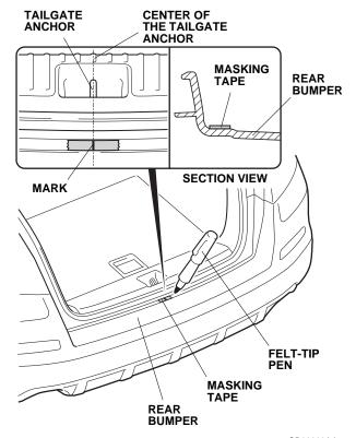
2. Align the rear bumper applique to the rear bumper, and check the rear bumper applique attaching position.
