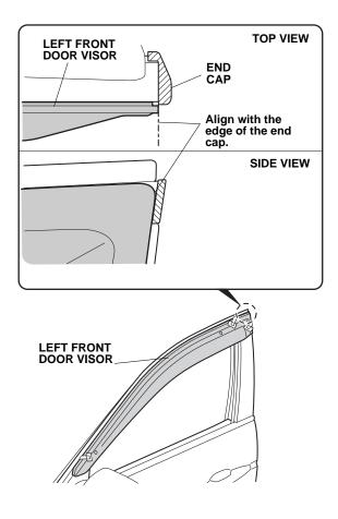
8. While holding the door visor up firmly, remove the adhesive backing in the order shown. Use your finger to push up each bracket so there is no gap between the brackets and the door sash.
