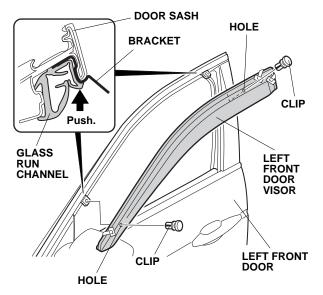
7. Align the door visor with the edge of the end cap.
