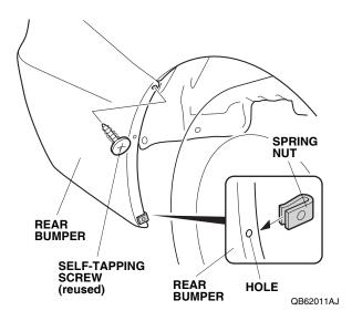
41. Install one spring nut over the hole in the rear bumper. Make sure to install the spring nut in the correct position and orientation. 42. Attach the right rear splash guard on the inner side of the right rear inner fender, and secure the right rear splash guard with two 5 x 25 mm self-tapping screws and one 5 x 30 mm self-tapping screw in the order shown below.
