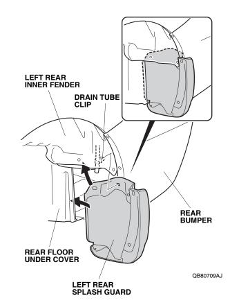
Secure the left rear splash guard with two 5 x 25 mm self-tapping screws and one 5 x 30 mm self-tapping screw in the order shown below.
