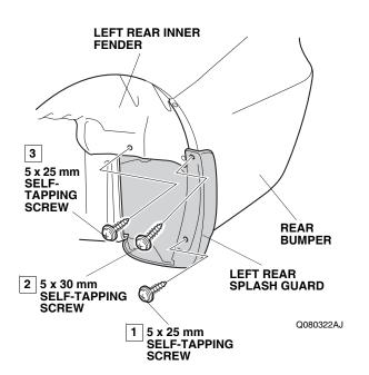
20. Secure the left rear splash guard with two new clips. Go to step 32.
