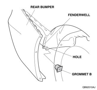
40. Reinstall the rear bumper onto the retaining tabs, and reinstall one self-tapping screw.
