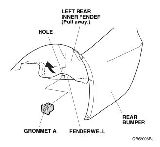
25. Pull the rear bumper away from the body, and release the seven retaining tabs.
