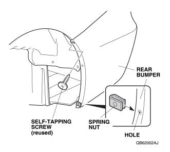
17. Install one spring nut over the hole in the rear bumper. Make sure to install the spring nut in the correct position and orientation. 18. Attach the left rear splash guard on the inner side of the rear floor under cover and the left rear inner fender, and install the drain tube clip to the left rear splash guard.
