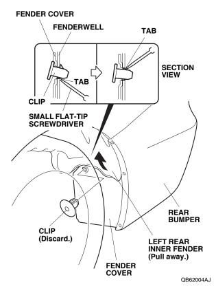
23. Remove the fender cover (one drain tube clip).
