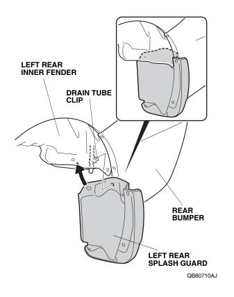
30. Secure the left rear splash guard with two 5 x 25 mm self-tapping screws and one 5 x 30 mm self-tapping screw in the order shown below. NOTE: Make sure there is no gap between the left rear splash guard and the bumper. If there is a gap, loosen the self-tapping screws, hold the splash guard against the bumper, and retighten the screws.
