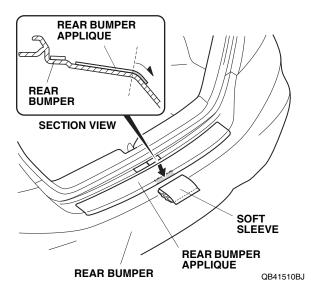
12. Use the soft sleeve to adhere the rear bumper applique to the lower section as shown.
