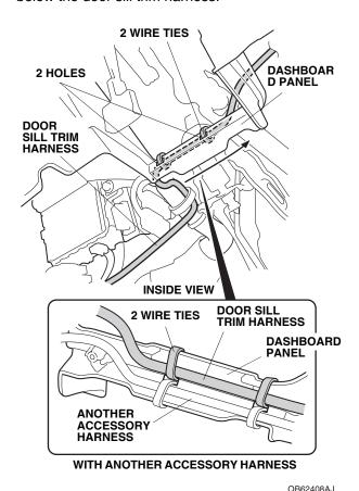
27. Route the door sill trim harness toward the passenger side of the vehicle, and secure it to the vehicle frame with one wire tie.
