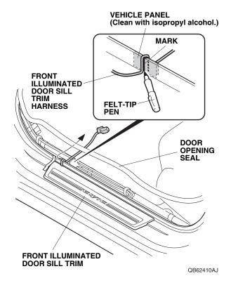
41. Using isopropyl alcohol on a shop towel, clean the vehicle panel around the harness, then use a felt-tip pen to mark the vehicle panel at the harness.
