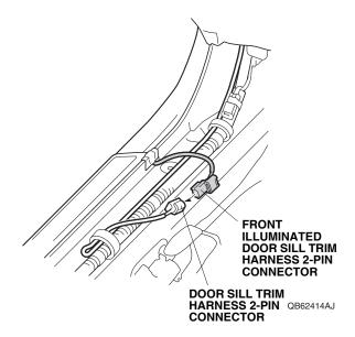
51. Bundle up the excess front illuminated door sill trim harness, and secure it to the vehicle harness with one wire tie with holder.
