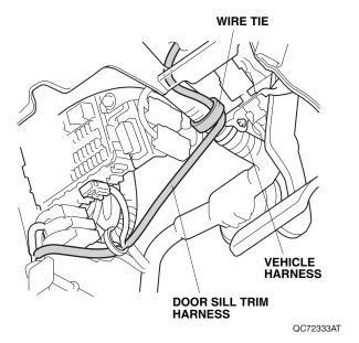
26. Secure the door sill trim harness to the holes in the dashboard panel with two wire ties. If another accessory harness is already attached to the dashboard panel, route and attach the other harness below the door sill trim harness.
