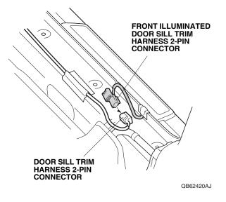
66. Bundle up the excess front illuminated door sill trim harness, and secure it to the vehicle harness with one wire tie with holder.
