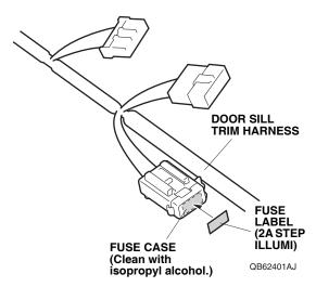
12. Attach the fuse label (2A STEP ILLUMI) to the door sill trim harness fuse case.
