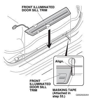
62. Attach the front illuminated door sill trim to the vehicle panel by removing three adhesive backings in the order shown and pressing on the trim firmly with your hands.
