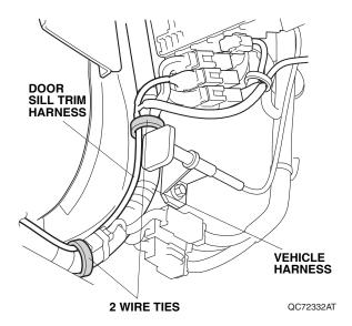
24. Continue to route the door sill trim harness along the vehicle harness, then loop the connector back to the measurement shown. Secure the door sill trim harness to the vehicle harness with one wire tie.
