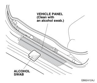
46. Position the front illuminated door sill trim on the vehicle panel and align it with the masking tape.
