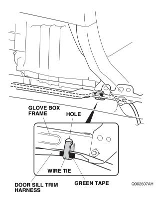
31. Secure the door sill trim harness to the glove box frame with one wire tie.
