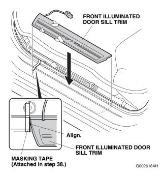
47. Attach the front illuminated door sill trim to the vehicle panel by removing three adhesive backings in the order shown and pressing on the trim firmly with your hands.
