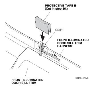
50. Plug the front illuminated door sill trim harness 2-pin connector into the door sill trim harness 2-pin connector.
