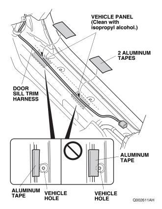
35. Secure the door sill trim harness to the vehicle panel with two aluminum tapes.
