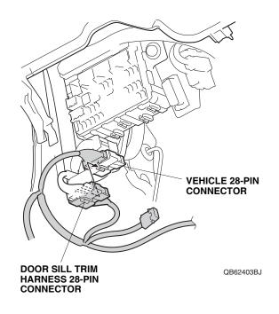
21. Attach the door sill trim harness fuse case to the bottom of fuse box.
