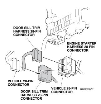
15. Plug the engine starter harness 28-pin connector into the vehicle 28-pin connector. Attach the connectors and clip on the engine starter harness as shown. Go to step 21.
