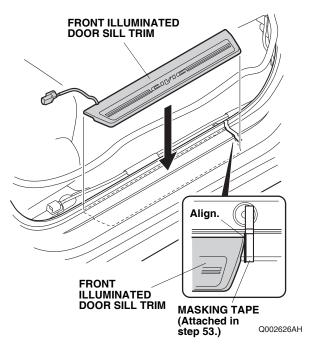
55. Route the front illuminated door sill trim harness over the vehicle panel of the door opening seal.
