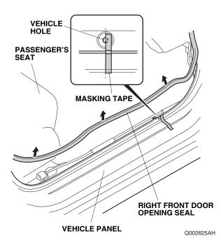
53. Attach a strip of masking tape to the vehicle panel at the location shown.
