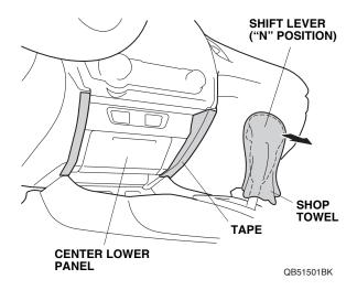
10. Remove the center lower panel (two self-tapping screws, four clips, and unplug the vehicle connectors, if equipped).
