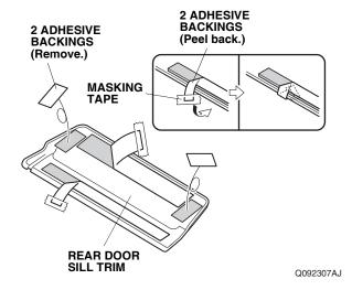
71. Position the rear door sill trim with the masking tape.
