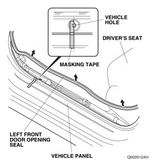
38. Attach a strip of masking tape to the vehicle panel at the location shown.
