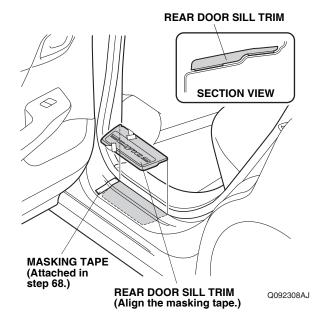
72. Attach the rear door sill trim to the vehicle panel by removing two adhesive backings and pressing on the trim firmly with your hands.
