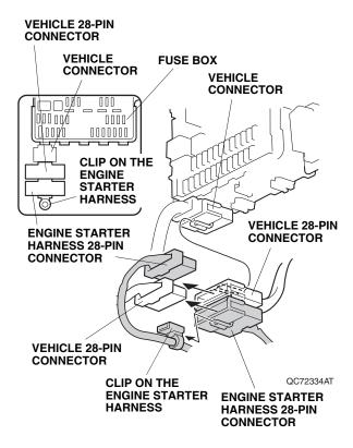
14. Plug the door sill trim harness 28-pin connector into the engine starter harness 28-pin connector. Plug the vehicle 28-pin connector into the remaining door sill trim harness 28-pin connector, and attach them to the vehicle 28-pin connector.
