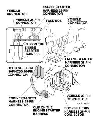
19. Attached to the bottom of the fuse box, locate the vehicle 28-pin connector. Unplug the vehicle 28-pin connector and plug it into the door sill trim harness 28-pin connector. Plug the door sill trim harness 28-pin connector into the vehicle 28-pin connector.
