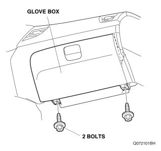
Open the glove box, push inward on the stops, and remove the glove box.
