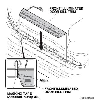
40. Route the front illuminated door sill trim harness over the vehicle panel of the door opening seal.
