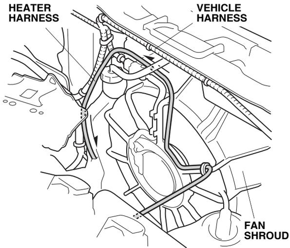
15. Using two black wire ties and three white wire ties, secure the heater harness to the fan shroud rib and vehicle harness.
