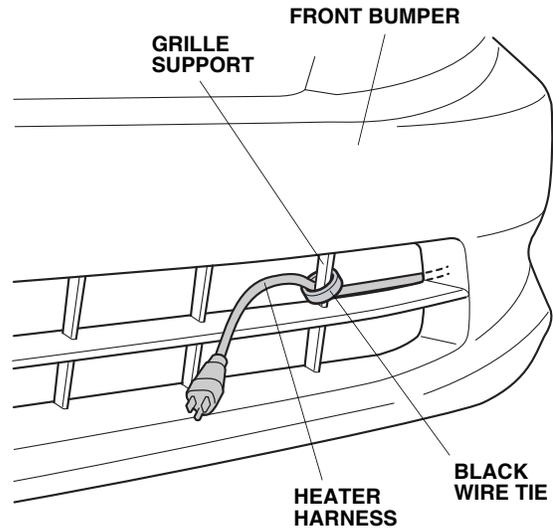
25. Attach the protective cap to the front bumper grille support, and plug the heater harness connector into the protective cap.
