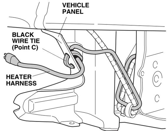
22. Using an additional black wire tie, secure the heater harness to the vehicle harness as shown.
