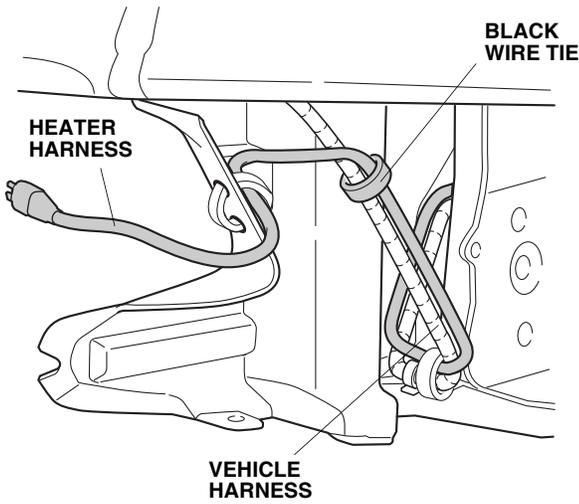
23. With the help of an assistant, route the heater harness through the grille opening in the bumper, then reinstall the front bumper.
