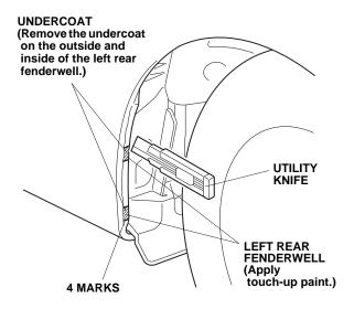
7. Apply touch-up paint to the area where the undercoat is removed, and allow it to dry thoroughly.
