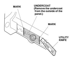
3. Remove the bolt from the vehicle panel.
