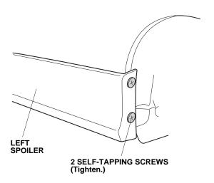
44. Tighten the bracket screw.
