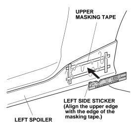
55. While holding the left side sticker to keep it from moving, use an applicator to remove any air bubbles under the left side sticker. Move the applicator in one direction only.
