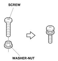
40. Using a Phillips screwdriver, securely tighten the screw into the clamp. Finger-tighten the washer-nut against the clamp. While holding the screw, tighten the washer-nut 90° clockwise with a 10 mm open end wrench.
