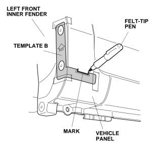
12. Carefully remove template B. Do not damage the template. It is also used for installing the right side spoiler.
