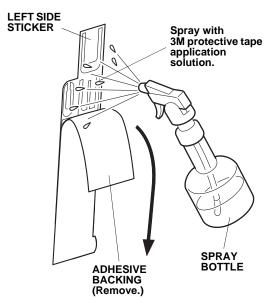
53. Spray the left side sticker with 3M protective tape application solution.
