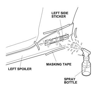
57. Use the applicator to remove any remaining air bubbles. Take care not to move the left side sticker out of the proper position. Move the applicator in one direction only.
