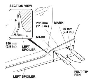
49. Attach masking tape to the left spoiler at the marks you made.
