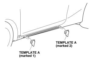
24. If the ambient air temperature is 15°C (60°F) or below, use a dryer to heat the surface of the rail to 15 - 40°C (60 - 104°F). The rail may not properly adhere to the vehicle otherwise.
