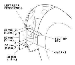
6. Using a utility knife, remove the undercoat in the areas shown.
