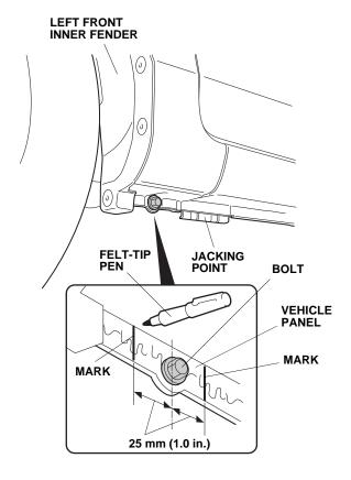
2. Using a utility knife, remove the undercoat between the marks.
