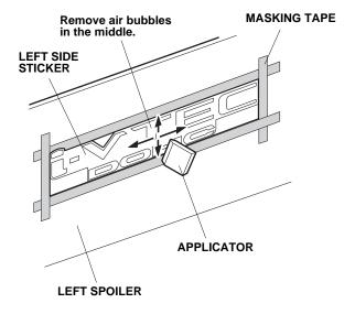
56. Spray the left side sticker again with 3M protective tape application solution. Remove the masking tape.
