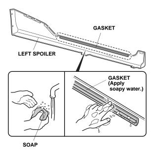
29. Align the gasket on the left spoiler to the rail. Insert the front end of the gasket to the rail first, then work toward the rear. Move the left spoiler gently up and down, and confirm that the gasket is installed securely to the rail.
