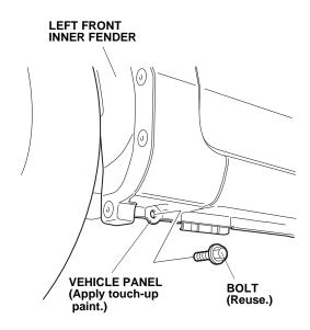
4. Apply touch-up paint to the area where the undercoat is removed. Allow it to dry thoroughly.
