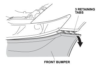
· Release five retaining tabs on each side.
