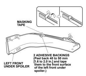
7. Install the left front under spoiler with one bumper clip.
