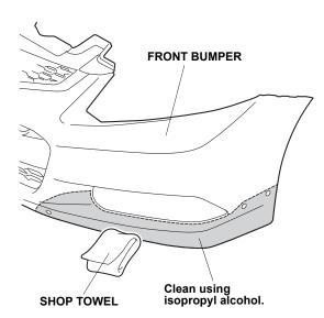
6. Peel back about 40 to 50 mm (1.6 to 2.0 in.) of adhesive backing from each adhesive strip, and tape the ends to the front surface of the left front under spoiler.
