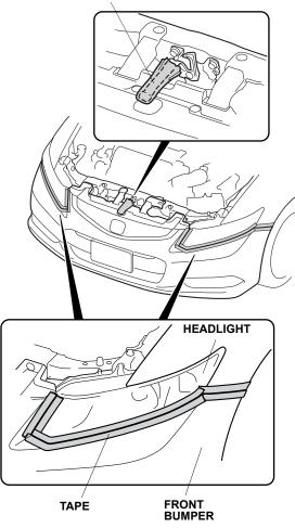
Remove the four self-tapping screws, ten short clips, and two long clips.
