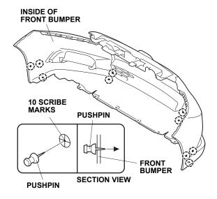
3. While wearing eye protection, drill the 10 pierced marks with a 3 mm drill bit, then enlarge the holes with a 10 mm drill bit.
