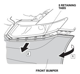
With the help of an assistant, remove the front bumper (two hex bolts, two clips, and unplug the vehicle connectors). Place the front bumper on a blanket to prevent damage.
