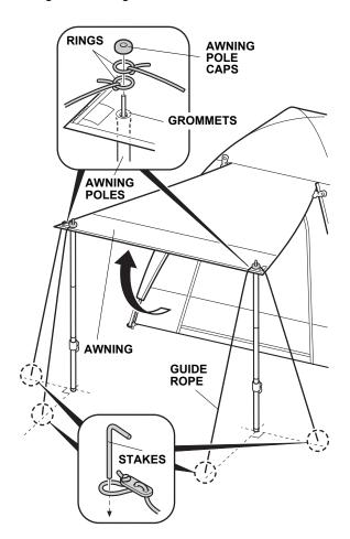
17. Pull the awning tight, adjust the height of the awning using the telescopic pole, and secure the awning to the ground using an additional stake and guide rope. Secure the other pole using the same procedure. If necessary, adjust the guide rope length using the adjuster on the rope.
