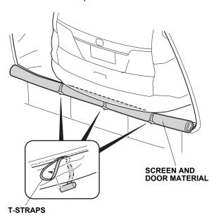
8. Stretch the bottom elastic strap across the rear face of the bumper. Make sure the tent material is tight against the rear face of the bumper, with the exhaust pipe outside the tent. Go outside of the tent, and make sure the exhaust pipe is outside.
