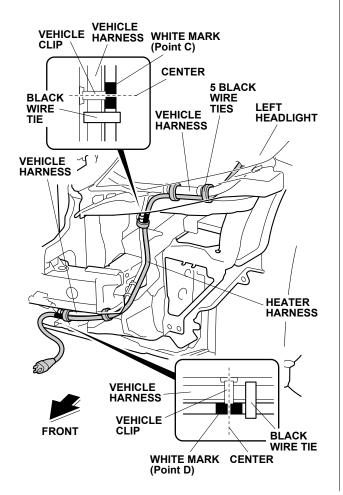
46. Near the fuse box, secure the heater harness to the vehicle harness with two black wire ties.
