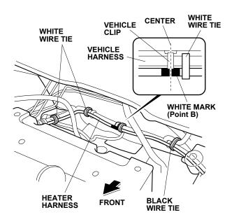
42. Route the heater harness to the driver's side of the fuse box as shown.
