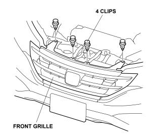
11. Using a flat-tip screwdriver, release the four clips from the bottom of the front grille.
