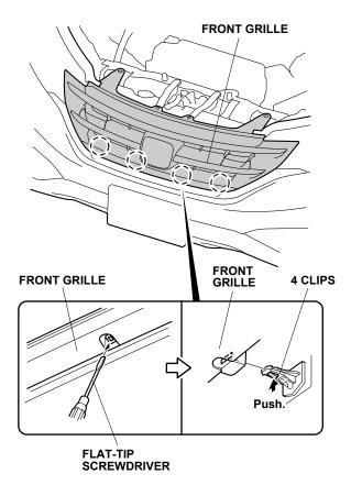
12. Using a long blade flat-tip screwdriver, release the one clip and the two retaining tabs from each side of the front grille.
