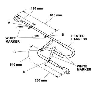
39. Plug the heater harness connector to the engine block heater. Make sure that the heater harness connector is properly installed.
