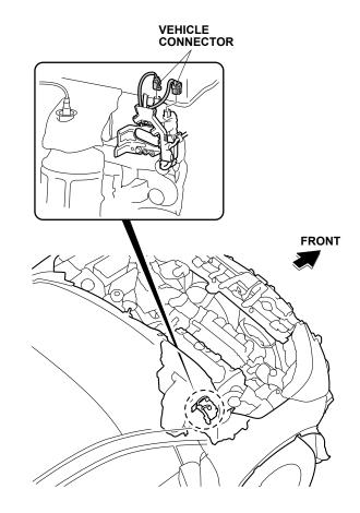
35. Release the vehicle harness holder from the vehicle bracket (two hooks).
