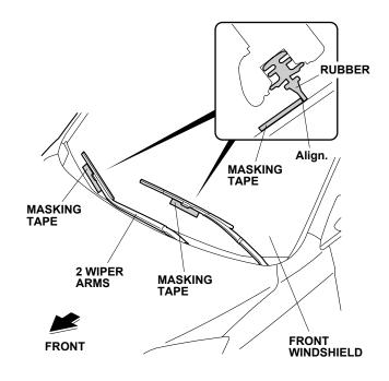
15. Remove the two windshield wiper arms (two caps and two nuts). Wiper arm nut torque is 29.4 N⋅m (21.6 lbf⋅ft).
