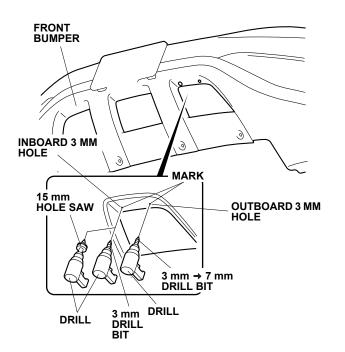
50. Using a 7 mm drill bit, enlarge the outboard 3 mm hole to 7 mm. Using a 15 mm hole saw, enlarge the inboard 3 mm hole to 15 mm.
