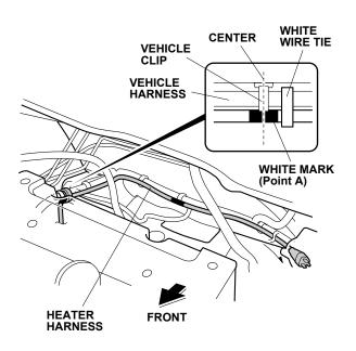
41. Align the mark at the point B with the vehicle clip, and secure the heater harness to the vehicle harness with three white wire ties and one black wire tie as shown.
