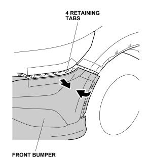
• Attach masking tape to the front bumper in the area shown.
