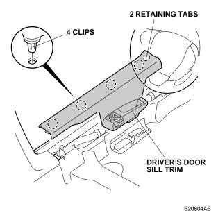
2-Door: Two retaining tabs and six clips.
