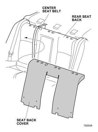
10. Secure the three hook-and-loop fasteners to the rear seat back. Raise the rear seat back and lock it to its original position.
