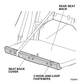
11. Insert the seat back cover under the headrest guides. Pull down the armrest, secure the hook-and-loop fastener to the rear seat back.
