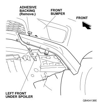
15. Using you hand, firmly press the left front under spoiler against the front bumper for 30 second.
