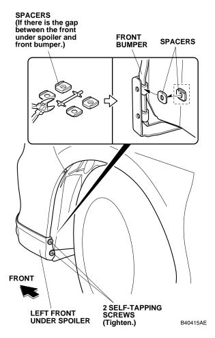
18. Turn the template over and repeat steps 2 through 17 to install the right front under spoiler on the right side of the vehicle.
