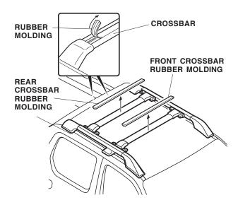
2. Insert two long T-bolts into each crossbar through the opening.
