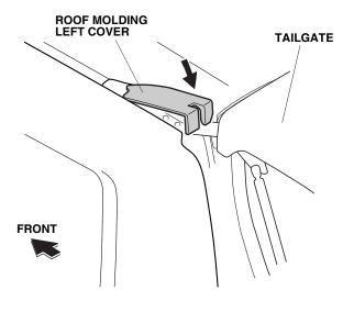
12. Reinstall the roof moldings back into the left roof channel using the two new roof molding clips installed in step 10.
