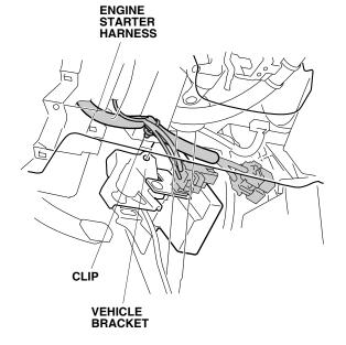
31. Route the engine starter harness relay block toward the right side of the vehicle.
