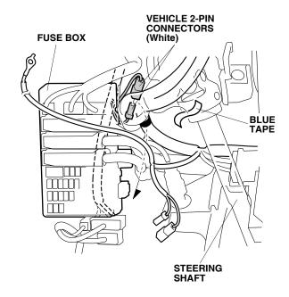
37. Plug the engine starter harness 2-pin connectors to the vehicle 2-pin connectors as shown.
