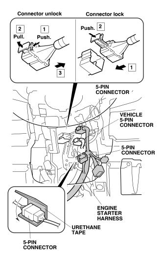
51. Plug the engine starter harness 5-pin connector into the vehicle 5-pin connector.
