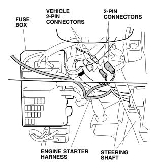
38. Route the engine starter harness 2-pin connectors behind the fuse box as shown.
