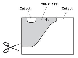
60. Align the template with edge of the black ceramic paint as shown, then secure the template to the windshield with masking tape.
