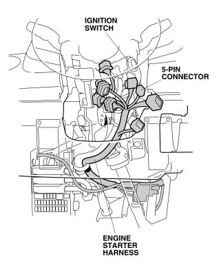
46. Unplug the vehicle 12-pin connector, and plug it into the engine starter harness 12-pin connector. Plug the remaining engine starter harness 12-pin connector into the turn signal switch.
