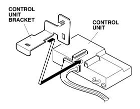
28. Secure the control unit to the vehicle bracket with a 6 mm flange nut.
