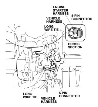
54. Unplug the vehicle 7-pin connector from the ignition switch, and plug the engine starter harness 7-pin connectors to the ignition switch and to the vehicle 7-pin connector.
