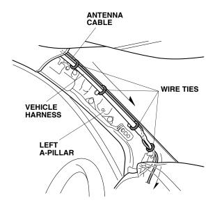
68. Secure the antenna cable to the vehicle harness with one wire tie.
