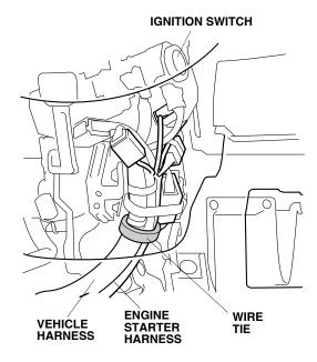
56. Adjust the steering wheel in, out, up, and down while you check the engine starter harness routing. If the harness is rubbing against the steering column bracket, check the installation and position of the wire ties installed in steps 53 and 55. **57.** Using two needle nose pliers, bend the antenna plate according to the drawing shown,
