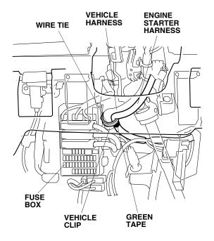
36. Locate and remove the blue tape from the vehicle 2-pin connectors (white), and unplug the vehicle 2-pin connectors as shown.
