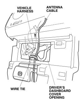
69. Route the antenna cable along the engine starter harness. Secure the antenna cable to the vehicle harness with the two wire ties that were loosely installed in step 44.
