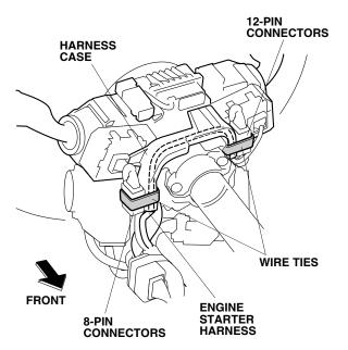
50. Unplug the vehicle 5-pin connector from the ignition switch, and plug the engine starter harness 5-pin connector into the ignition switch.
