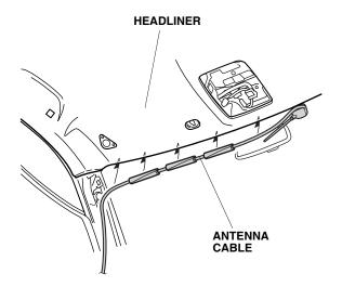
65. Clean the vehicle panel surface with isopropyl alcohol where the urethane tape will attach. Secure the antenna cable to the vehicle panel with one half of the urethane tape that you cut into two in step 40. Be careful not to crease the headliner.
