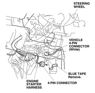
34. Secure the 4-pin connector to the vehicle harness with one wire tie.
