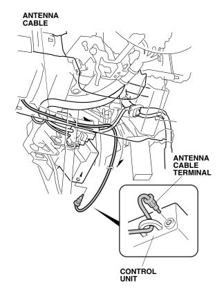
71. Secure the engine starter harness and antenna cable with one wire tie as shown.
