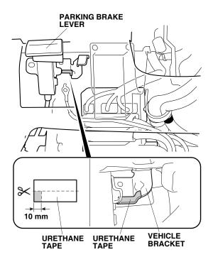
41. Clean the vehicle bracket surface with isopropyl alcohol where the urethane tape will attach. Attach the 10 mm piece of urethane tape to the vehicle bracket as shown.
