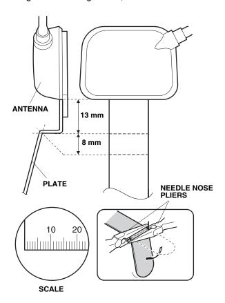
58. Starting at the antenna end of the cable, wrap three urethane tapes around the antenna cable at the measurements shown.
