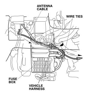
70. Route the antenna cable terminal toward the right side of the vehicle, and plug it into the control unit as shown.
