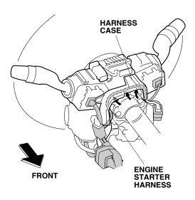
49. Secure the 12-pin and 8-pin connectors to the harness case with two wire ties.
