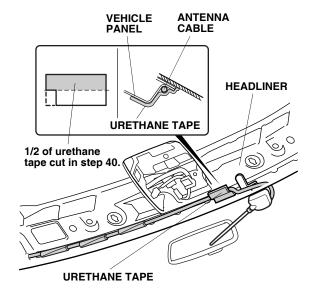
66. Clean the vehicle panel surface where the urethane tape will attach with isopropyl alcohol. Secure the antenna cable to the vehicle panel with the remaining part of the urethane tape you cut in step 40. Be careful not to crease the headliner.
