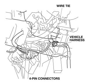
35. Align the green tape on the engine starter harness with the vehicle clip. Secure the engine starter harness to the vehicle harness with one wire tie.
