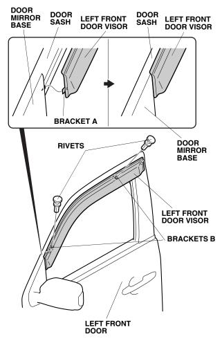
6. Align the holes in the brackets B with the holes in the left front door visor and secure it with two rivets.
