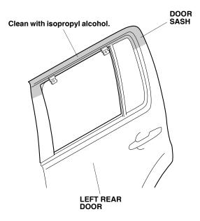
14. Align the holes in the brackets C to the holes in the left rear door visor and secure it with two rivets.
