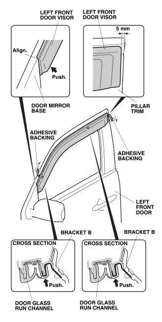
8. Remove the adhesive backings from the left front door visor.
