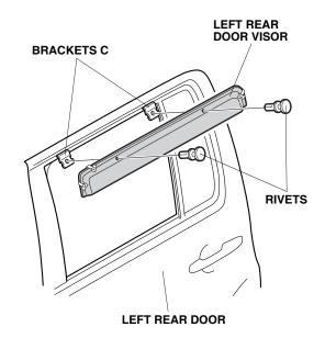
15. Adjust the position of the left rear door visor. Make sure there is no clearance between the bracket and the door sash.
