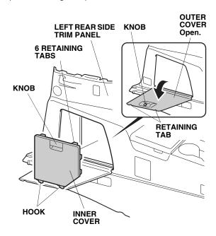
44. Pull the knob, and remove the inner cover from the left rear side trim panel (six retaining tabs and two hooks).
