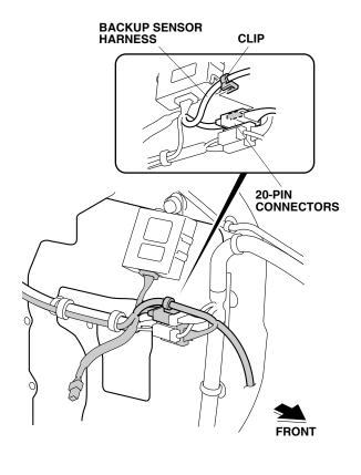
36. Route the backup sensor harness along the vehicle harness, and secure it to the vehicle harness with three wire ties.
