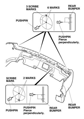
53. While wearing eye protection, drill the eight pierced marks with a 3 mm drill bit from the painted side of the rear bumper.
