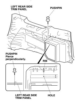
46. While wearing eye protection, drill a 3 mm hole at the pierced mark. Enlarge the 3 mm hole to 26 mm using a 26 mm hole saw.
