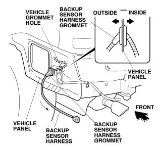
41. Slide the connector clip onto the backup sensor harness 6-pin connector, then install the connector clip into the vehicle panel hole.
