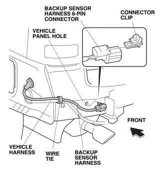
42. Secure the backup sensor harness to the vehicle harness with one wire tie.
