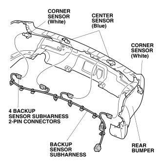
59. Secure the three backup sensor subharness clips to the three sensor clips as shown.
