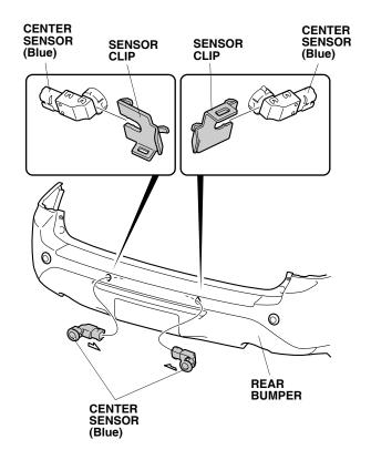
58. Plug the four backup sensor subharness 2-pin connectors into the four sensors.
