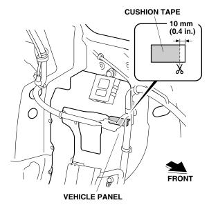
28. Using isopropyl alcohol on a shop towel, clean the vehicle panel where the cushion tape will attach. Attach the cushion tape to the vehicle panel in the area shown.
