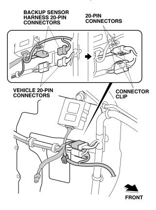
34. Attach the 20-pin connectors together using the connector clip.
