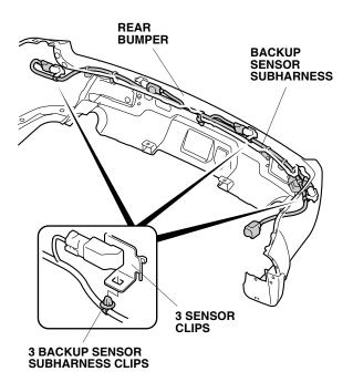
60. Secure the four backup sensor subharness clips to the four ribs on the rear bumper as shown.
