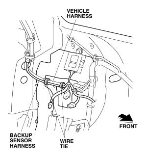
33. Unplug the vehicle 20-pin connector, and plug it into the backup sensor harness 20-pin connector. Plug the remaining backup sensor harness 20-pin connector into the vehicle 20-pin connector.
