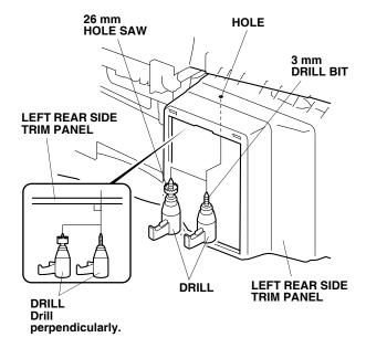
47. Install the switch into the 26 mm hole in the left rear side trim panel.
