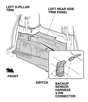
51. Bring the left rear side trim panel into position, plug the backup sensor harness 3-pin connector into the switch, and reinstall the left rear side trim panel.
