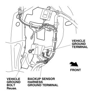
38. Route the backup sensor harness along the vehicle harness, and secure it to the vehicle harness with three wire ties.
