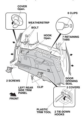
14. Pull away the weatherstrip and door opening seal at the front and rear of the left rear side trim panel. Remove the left rear side trim panel. 15. Remove the cover from the left D-pillar trim (six retaining tabs).
