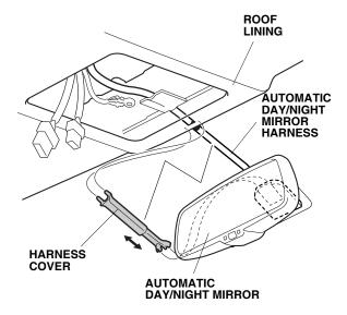
15. Adjust the harness cover to fit under the roof lining.
