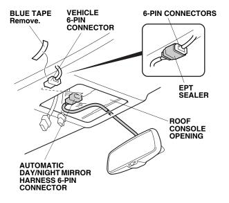
12. Wrap an EPT sealer around the 6-pin connectors.
