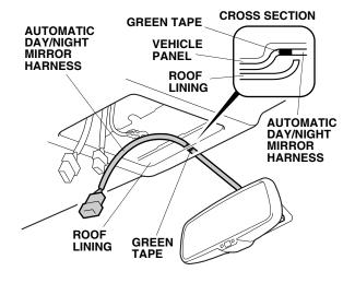
Locate the vehicle 6-pin connector and remove the blue tape. Plug the automatic day/night mirror harness 6-pin connector to the vehicle 6-pin connector.
