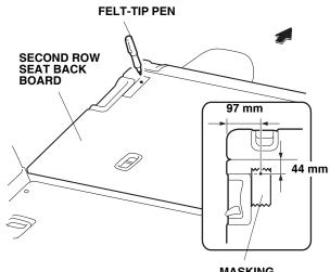
MASKING TAPE 13. While wearing eye protection, drill the marked locations with a 3 mm drill bit, and then with a 5 mm drill bit. Drill through the hard board and the sheet metal. To prevent damage to the seat, wrap tape around the drill bit 25 mm from the tip as shown.
