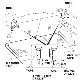
7. Enlarge the holes with a 10.5 mm drill bit. To drill through the hard board only, wrap tape around the drill bit 10 mm from the tip as shown.
