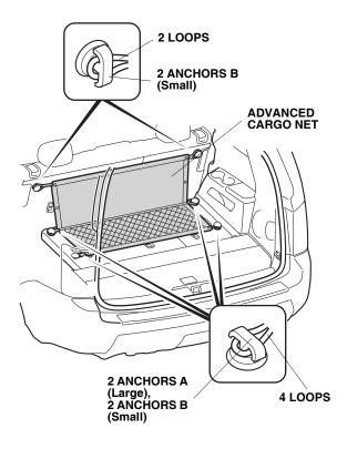
20. Attach six loops on the advanced cargo net to two anchors A (Large) and four anchors B (Small) on the second and third row seat back boards.
