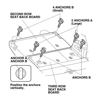
18. Install the four anchors B (Small) on the second and third row seat back boards into the holes made in steps 8 and 13.
