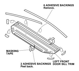
8. Remove the remaining adhesive backings.
