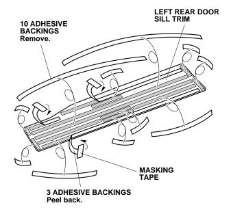
19. Remove the remaining adhesive backings.
