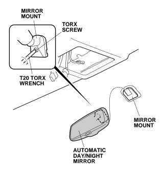
Route the automatic day/night mirror harness as shown. Plug the automatic day/night mirror harness 7-pin connector to the automatic day/night mirror.
