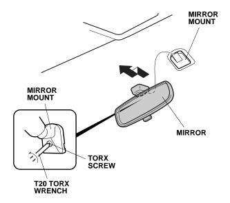
6. Install the automatic day/night mirror on the mirror mount as shown, and tighten the torx screw.
