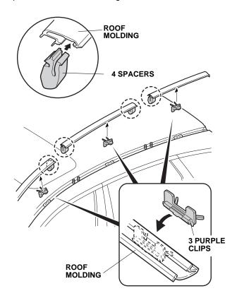
15. Reinstall the cut pieces of roof molding to the vehicle.
