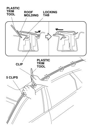
Pull the roof molding toward the outside of the vehicle to release the locking tabs, press the locking tabs towards the inside of the vehicle, and remove the roof molding from the vehicle. When removing the roof molding, start from the rear of vehicle and work toward the front. 4. Release the pin.
