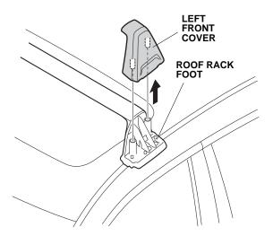
23. Remove four TORX nuts. Remove the front roof rack.
