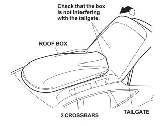
Open the roof box. Slide the plate forward or backward until the holes in the plate are over the front roof rack crossbar. The plate is located near the front of the roof box.
