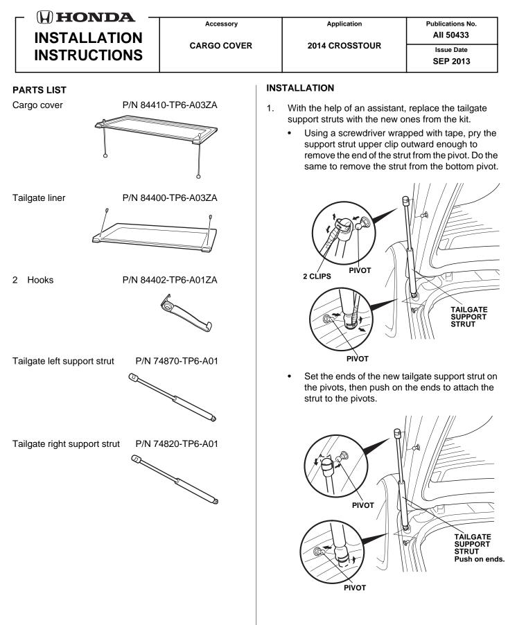
Repeat this procedure to install the tailgate support strut on the other side of the vehicle. 2. Remove the washer-screw from the tailgate left panel. Open the cover on the hook, then use the washer-screw to install the hook to the tailgate panel. Repeat this step to install a hook on the right side.
