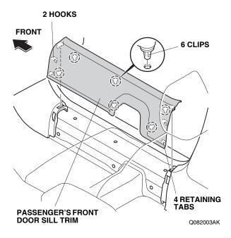
3. Pull away the door opening seal, and remove the passenger's kick panel (two clips).
