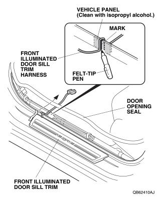
35. Using isopropyl alcohol on a shop towel, clean the vehicle panel around the harness, then use a felt-tip pen to mark the vehicle panel at the harness.
