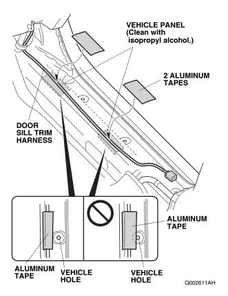
Secure the door sill trim harness to the vehicle panel with two aluminum tapes.
