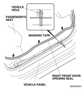
47. Attach a strip of masking tape to the vehicle panel at the location shown.
