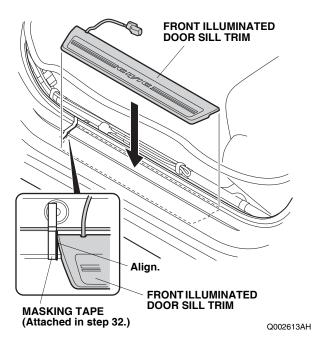
34. Route the front illuminated door sill trim harness over the vehicle panel of the door opening seal.
