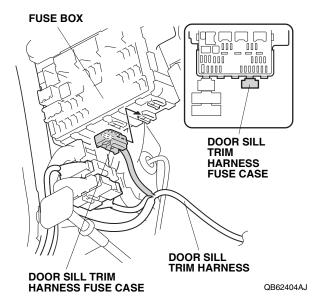
Secure the door sill trim harness to the vehicle harness with one wire tie.
