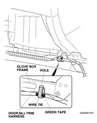
25. Secure the door sill trim harness to the glove box frame with one wire tie.
