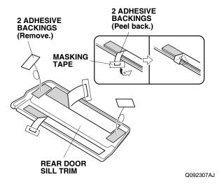
65. Position the rear door sill trim with the masking tape.
