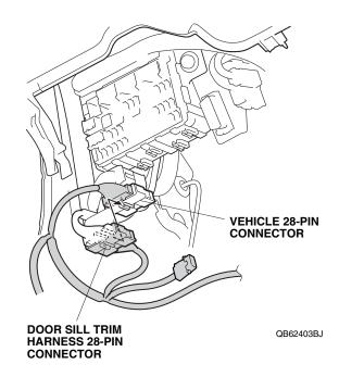
15. Attach the door sill trim harness fuse case to the bottom of fuse box.
