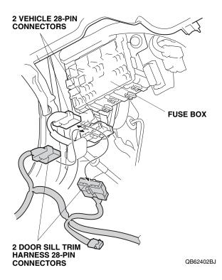
14. Attach the door sill trim harness 28-pin connector to the vehicle 28-pin connector.
