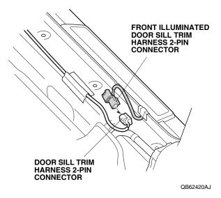
60. Bundle up the excess front illuminated door sill trim harness, and secure it to the vehicle harness with one wire tie with holder.
