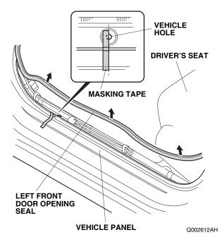
32. Attach a strip of masking tape to the vehicle panel at the location shown.
