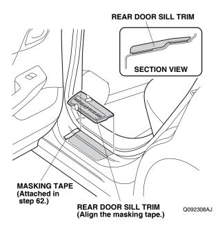
66. Attach the rear door sill trim to the vehicle panel by removing two adhesive backings and pressing on the trim firmly with your hands.
